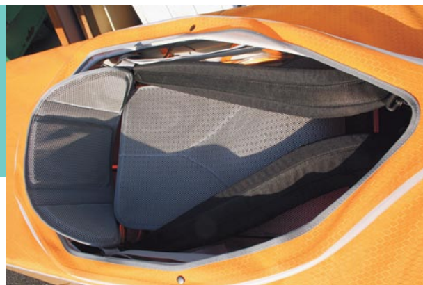
The seat has an inflatable forward end to provide leg support and padded thigh-brace straps.
